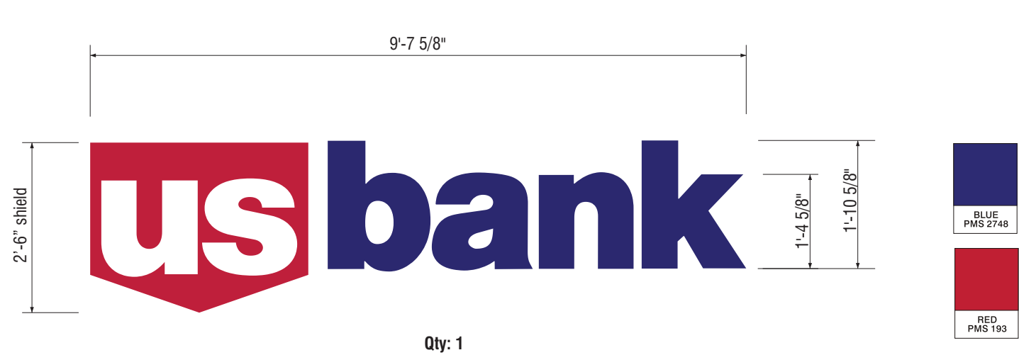
① Proposed Channel Letters & Logo - Remote Raceway Scale: 1/2" = 1' - 0" 24.10 sf
